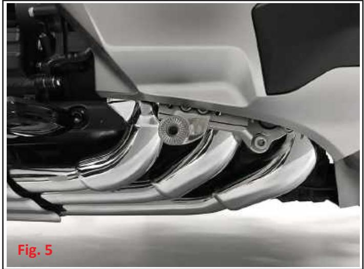
8. Install the engine cover. Start with the front lower corner first, ensuring the plastic hook is engaged correctly. then pop the center dart into place and reinstall the screws. (Fig.5)
